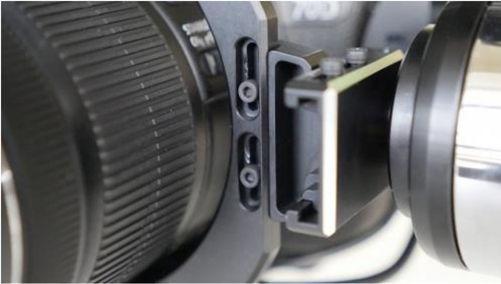
Locking position for the hot shoe cover
