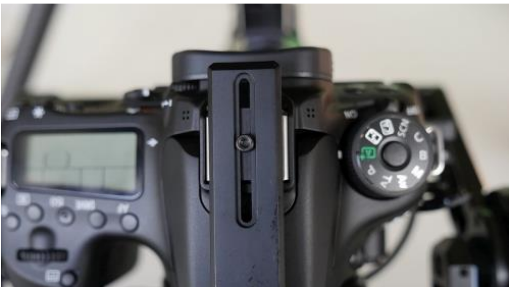
Locking position for the hot shoe Housing
